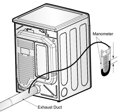
MAXIMUM STATIC PRESSURE IN WATER COLUMN
